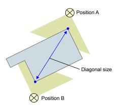
**Figure 10:** Measuring the diagonal size of a building footprint using data from two different scan positions, labelled A and B. Neither position can see the other corner, and while you might be able to place the scanner so it can see both corners, or at least, their edges, the scanner will not be able to see both walls for both corners at the same time, which is needed to find the corner precisely. Time to register.
