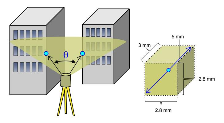
**Figure 3:** Measuring the space between two buildings. The diagonal error is swiftly computed from the specifications and the measurement situation.
