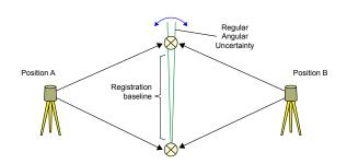
**Figure 11:** Registration involves comparing collections of points from one position to collections of points of a second position. The relative error is minimised under the presumption that the shared object from which the points are measured has not moved between the data collection events. The residual registration error tends to be smallest where registration algorithm checks, so the geometry (relative placement) of the patches used matter.
