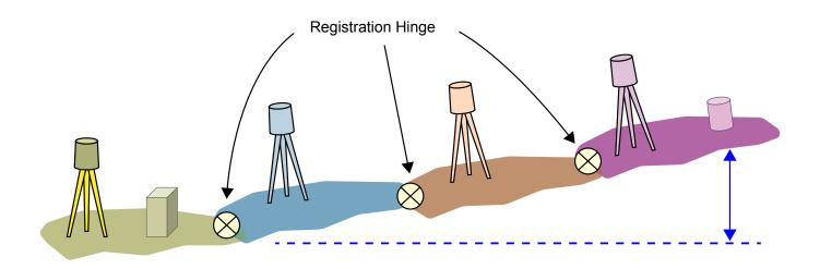
**Figure 12:** When the objects being scanned are all low, one might imagine that a long vertical baseline is unimportant. After all, nothing that is being measured is at any kind of height. Unfortunately, this is untrue. Registration errors can be very large even in flat land.
