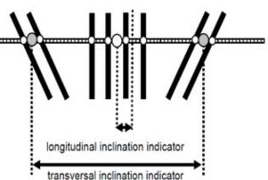
**Figure 2:** Leica Geosystems tilt sensors are also based on using a small line camera, much like the angular encoders. Much like the angular encoders, their sensitivity is very high, less than 1 arc second.
