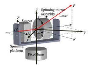
**Figure 7:** Figure underlying the mathematical model used in the NIST paper [1], as displayed in the paper. Notice the base of the scanner is labelled "Fixed".
