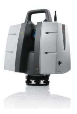
**Figure 1:** The Leica ScanStation P40, a survey grade laser scanner, with integrated tilt sensor, mounted on a surveying tribrach. The tribrach has three little wheels to allow fine levelling.
