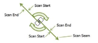
**Figure 18:** A close inspection of the scanning seam shows a deviation between the front face and the back face of the scan, and is colloquially known as a "scanning corkscrew".
