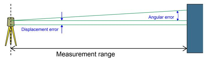
**Figure 5:** Bounding the accuracy of a point at a range of more than a few meters forces a brutal limit on the angular error of a point through the cruel lever of range, unlike displacement error.
