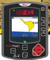
The graphical overview on PowerDigger Lite gives you information of the exact height and slope you have keyed in. All buttons and necessary functions are arranged logically resulting in very straight forward operation. PowerDigger Lite offers you the flexibility to work with an existing height or laser reference.
