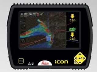
Display of the current snow depth on the machine display enables autonomous working
