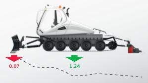
Three-point measurement under the clearing plough reduces the risk of collision
