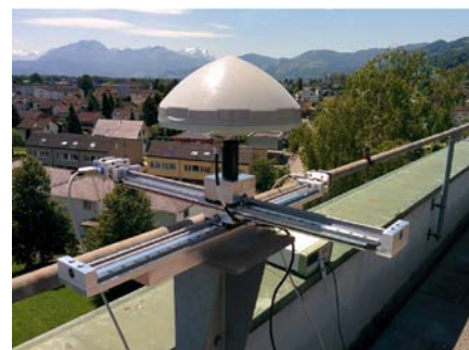
Figure 11: Dynamic platform on top of roof of building 03 in Heerbrugg Switzerland.
